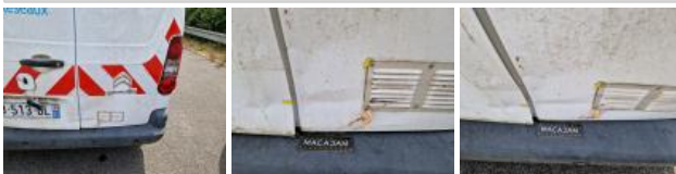
Shutter / cover R, Missing, Replace
