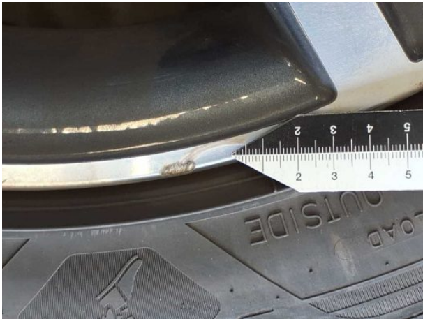
Damage #8: 2nd wheel set: 1 alloy rim (Im Fahrzeug liegend) - Scratched - Loss in value
