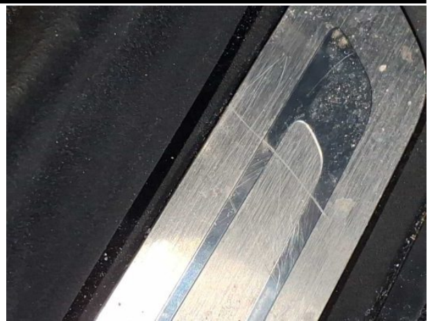
Damage #3: Trim / covers: Trim / covers (Einstiegsleiste) - Scratch(es) - Replace
