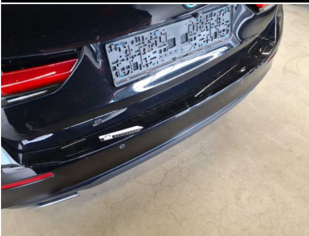
Damage #10: Rear bumper: Bumper with Parktronic - Dent / paintcoat damage - Repair and paint
