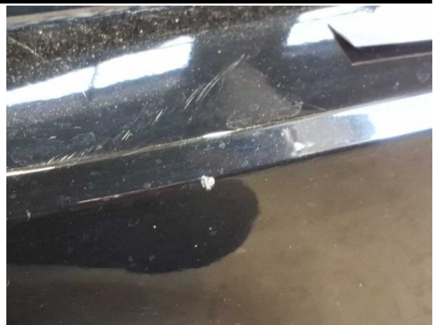
Damage #10: Rear bumper: Bumper with Parktronic - Dent / paintcoat damage - Repair and paint
