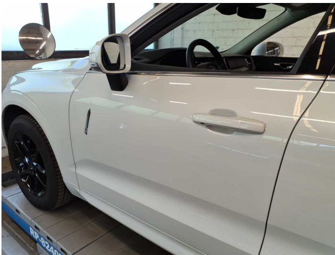
Damage 1: Door - front left side: Door (3 stk) - dent(s) - Smart repair
