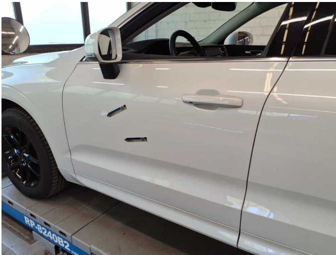
Damage 1: Door - front left side: Door (3 stk) - dent(s) - Smart repair
