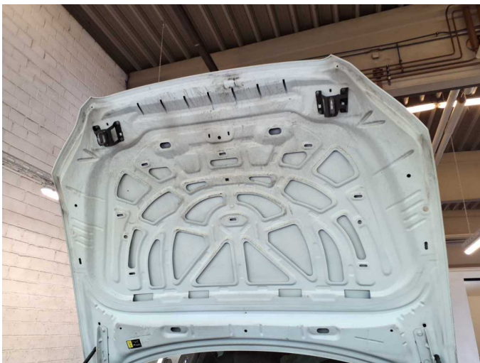
Damage 2: Bonnet: Insulation lining - Missing - Replace
