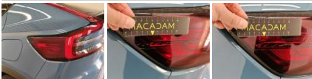
Rear light L, Scratch(es), Replace
