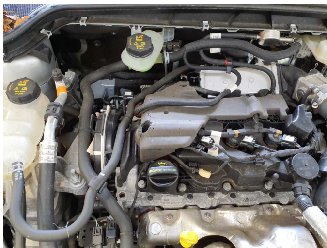
Damage 2: Misc.: Misc. (Isolierung Motorabdeckung) - Damage caused by marten / rodent - Replace
