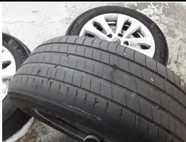
Damage #10: 2nd wheel set: 2 tyres - Worn - Replace
