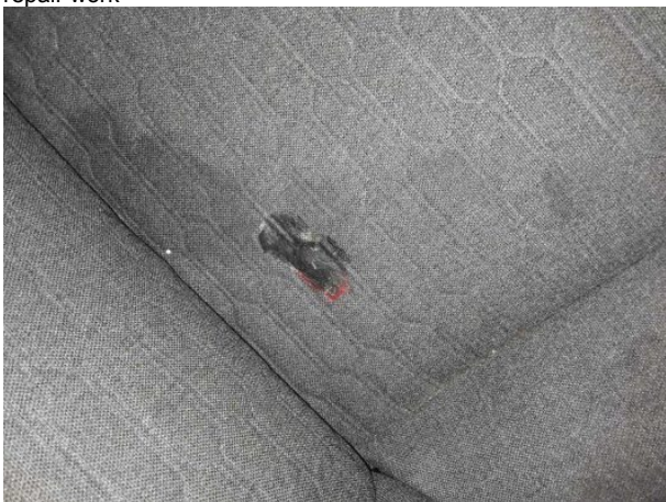
Damage #9: Seat - front: Seat cover - left side - Damaged - Replace
