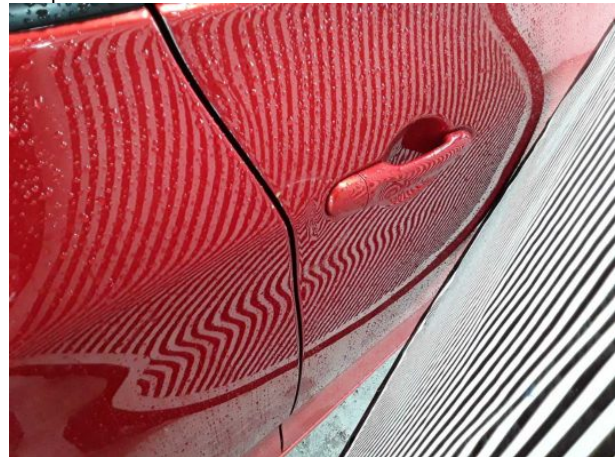
Damage #15: Door - front right side: Door - Deformed - Repair and paint
