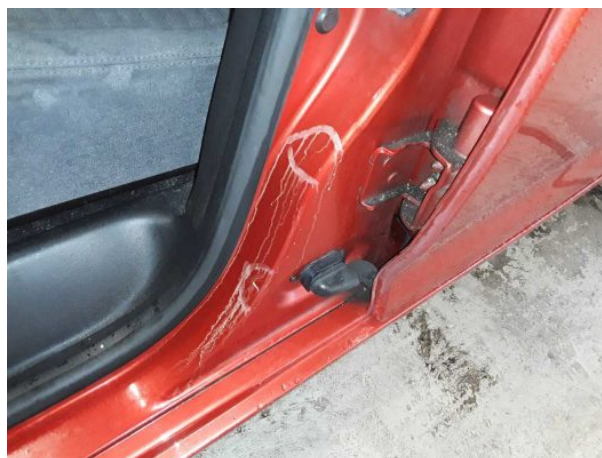
Damage #3: Sill - left side: Sill - Scratched - Smart repair
