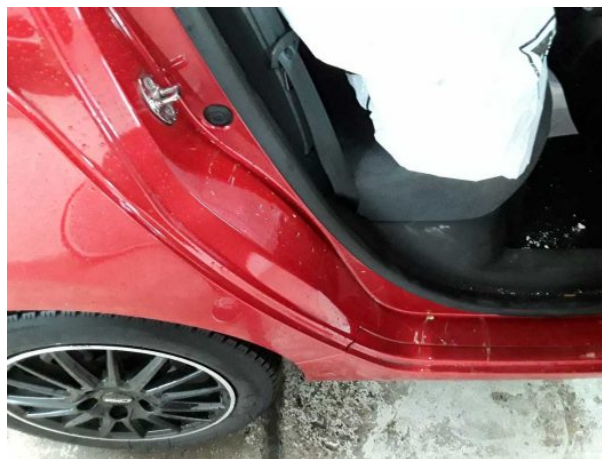
Damage #11: Side panel - rear right side: Sill - Dent / paintcoat damage - Repair and paint
