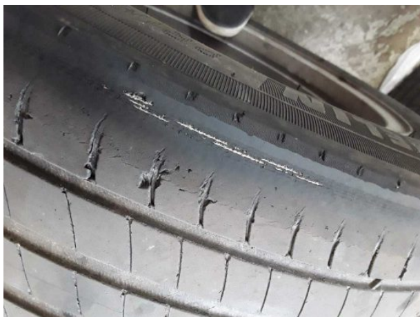
Damage #10: 2nd wheel set: 2 tyres - Worn - Replace
