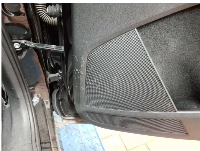
Damage 5: Interior: Interior - Scratch(es) - Loss in value
