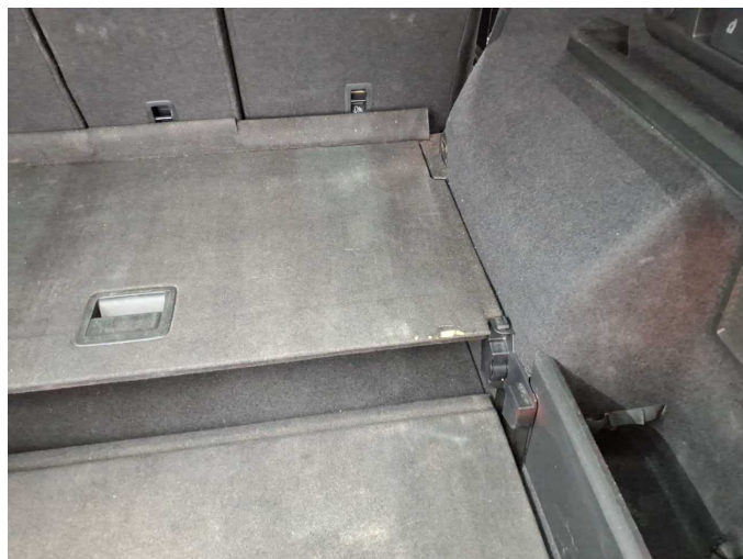
Damage 4: Interior: Cargo area floor - Broken / torn - Replace
