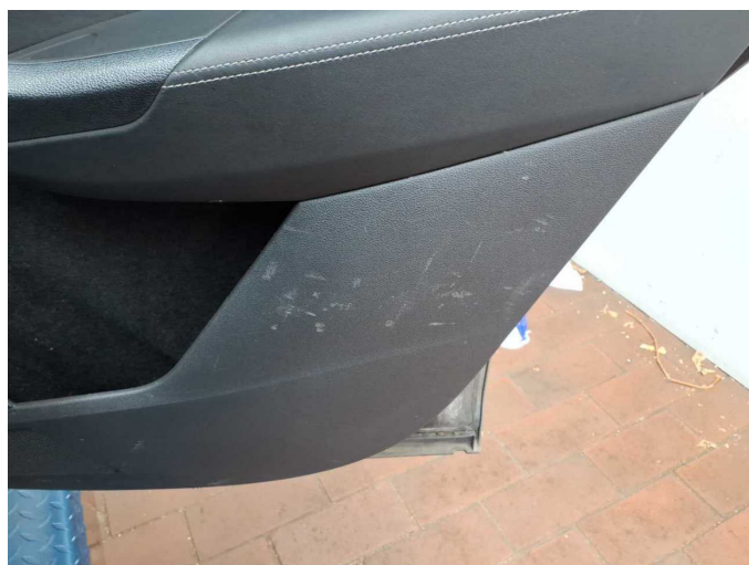
Damage 5: Interior: Interior - Scratch(es) - Loss in value
