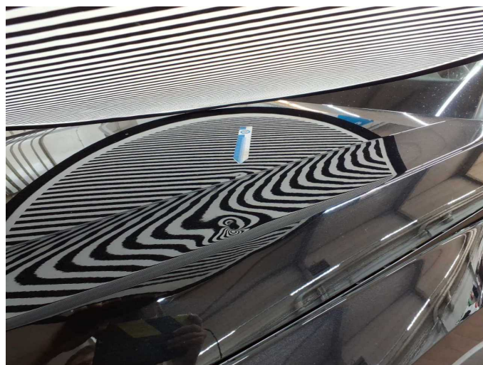
Damage 8: Bonnet: Bonnet - dent(s) - Repair and paint
