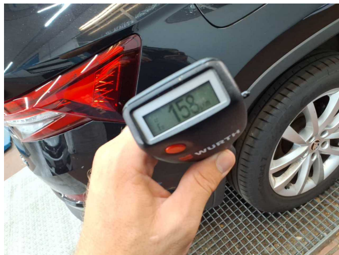
Repainting 1: Sill - right side
