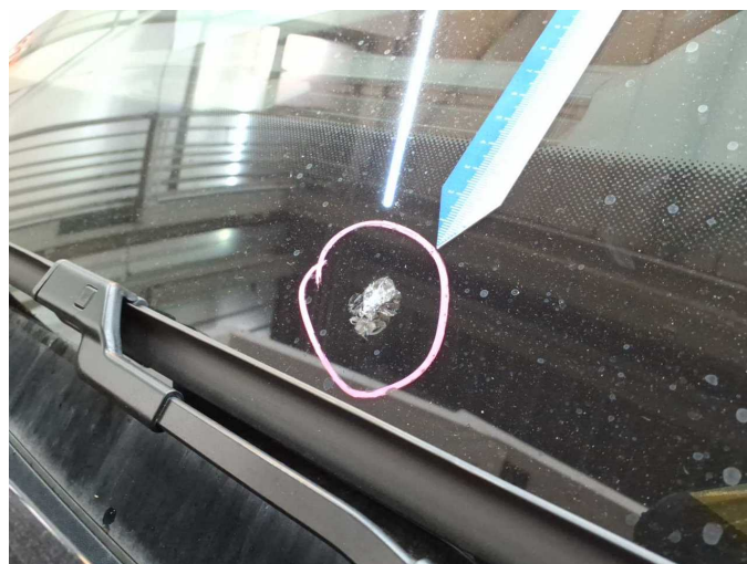
Damage 9: Vehicle glazing: Windscreen - Stone chips - Replace
