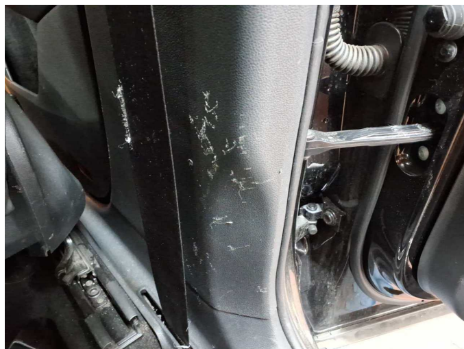
Damage 5: Interior: Interior - Scratch(es) - Loss in value
