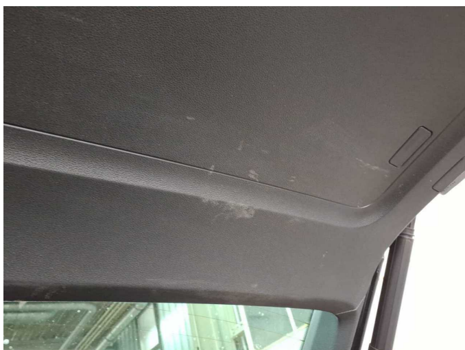
Damage 5: Interior: Interior - Scratch(es) - Loss in value
