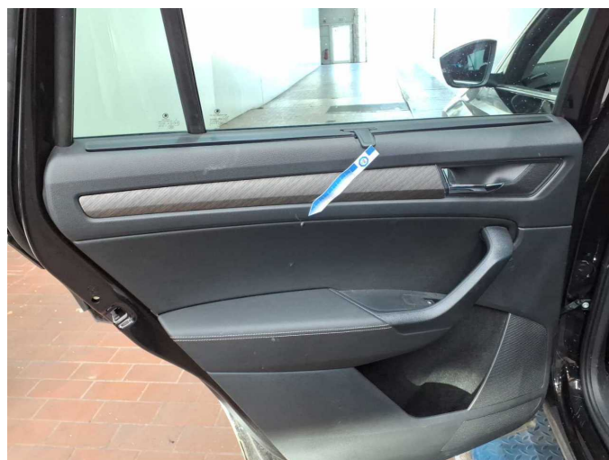
Damage 3: Trim / covers: Door trim - rear left side - Broken / torn - Smart repair
