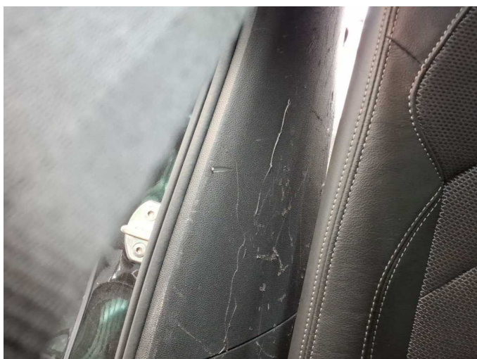
Damage 5: Interior: Interior - Scratch(es) - Loss in value
