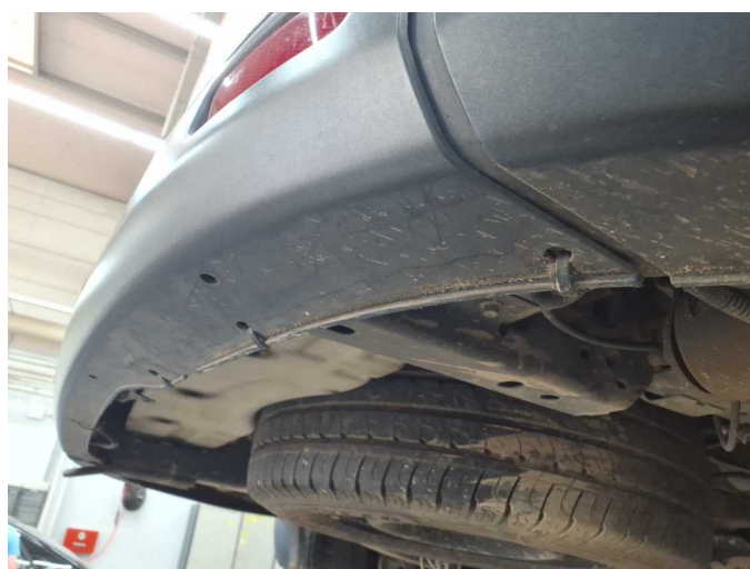
Damage 3: Rear bumper: Rear bumper - Loose - Repair
