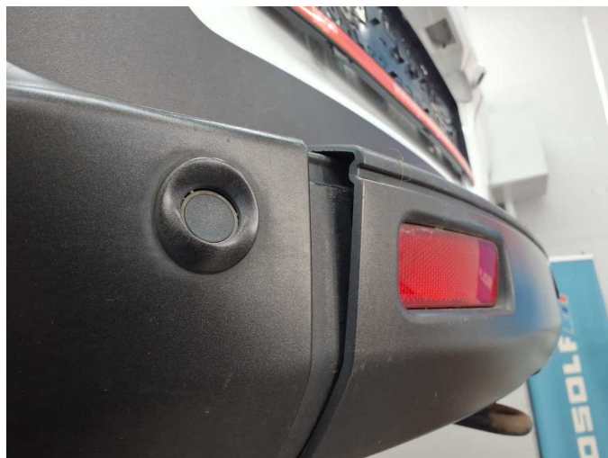
Damage 3: Rear bumper: Rear bumper - Loose - Repair
