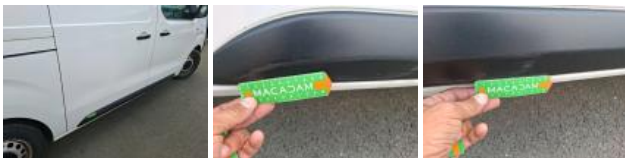
Outer sill R, Scratch(es), Paint
