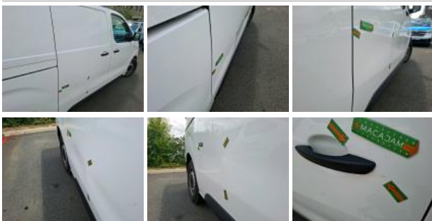
Door FR, Dent(s), Repair and paint (complete)
