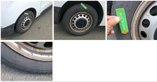
Tyre FR, Out of tolerance, Replace
