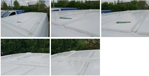
Load compartment roof, Dent(s), Repair and paint (complete)
