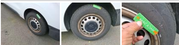
Tyre RL, Out of tolerance, Replace
