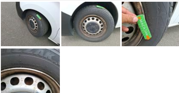
Tyre RL, Out of tolerance, Replace
