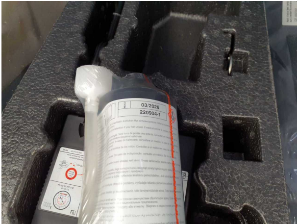
Damage #1: Equipment: Tirefit filler - Expired - Replace
