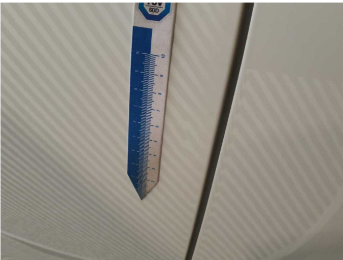
Damage 2: Door - rear right side: Door - dent(s) - Smart repair
