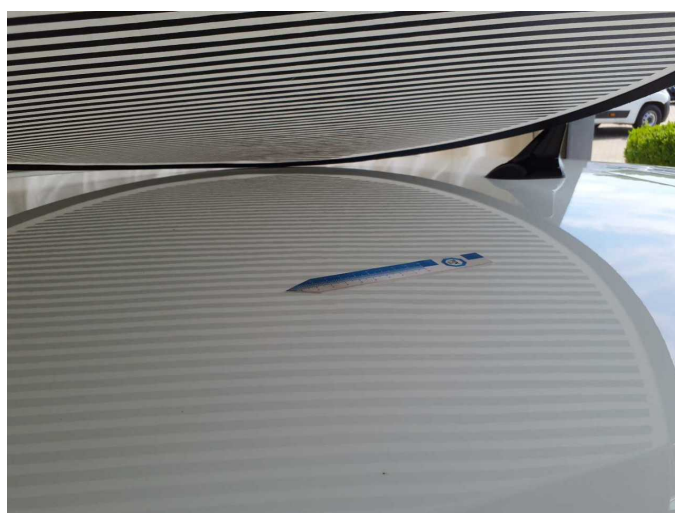
Damage 6: Roof: Roof (Wellig) - Paint defect - Repair and paint
