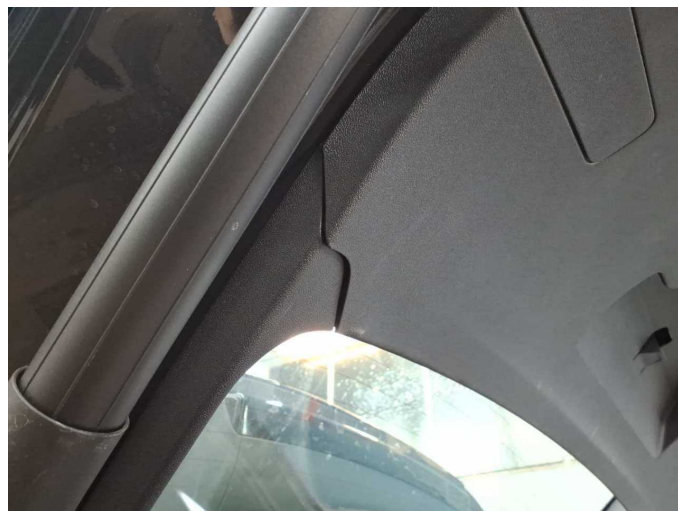
Damage 1: Trim / covers: Boot lid - interior trim - Loose - Repair
