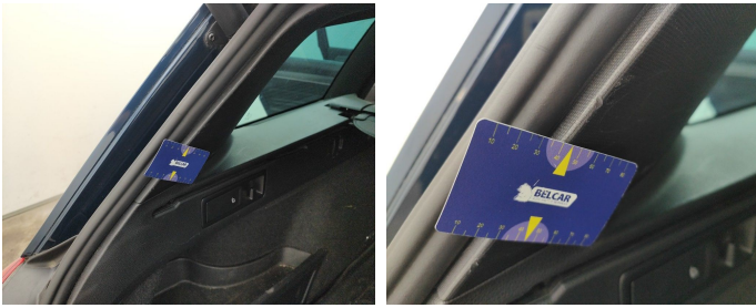
Trunk Compartment / Side Cover Left / Replace-scratch
