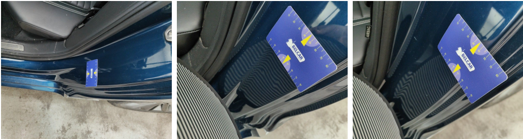
Rocker Panel Left // Smart Repair Medium-dent
