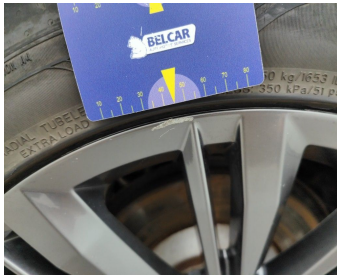
Wheel Alloy Rear Right // Repair-scratch
