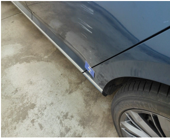
Wing Rear Left // Repair & Painting-scratch + dent
