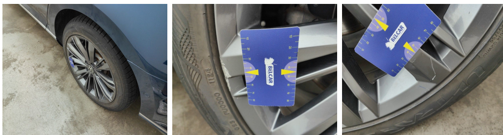
Wheel Alloy Rear Left // Repair-scratch
