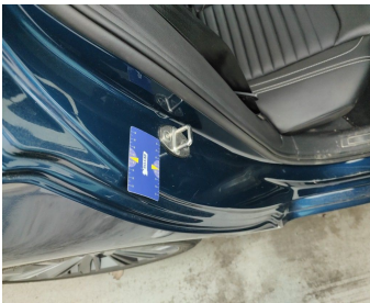
Rocker Panel Right // Smart Repair Medium-scratch + dent
