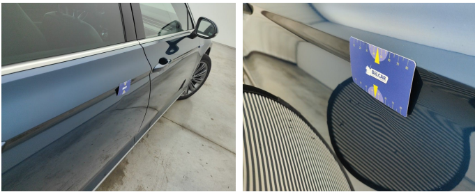
Door Rear Right // Smart Repair Medium-dent
