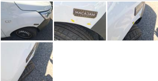
Bumper R, Deformed / Strained, Replace
