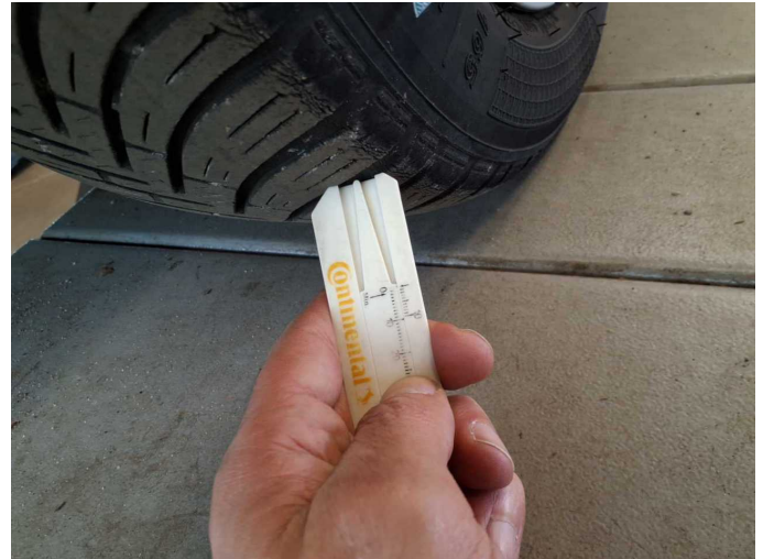
Damage 3: Wheel / tyres: Tyre - front (Rechts und links) - Does not meet the leasing specifications - Replace
