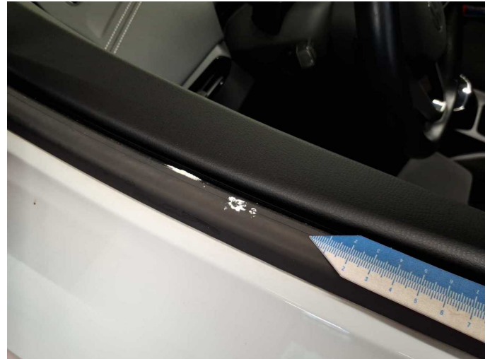
Damage 1: Door - front left side: Strip - outer - Soiled - Clean
