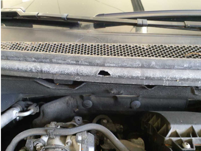
Damage 4: Cab: Insulation lining (+ Dichtung) - Damage caused by marten / rodent - Loss in value
