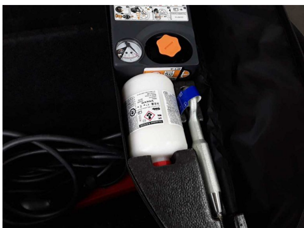
Damage #2: Equipment: Tirefit filler - Expired - Replace
