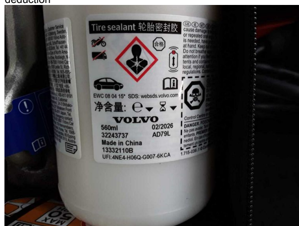
Damage #2: Equipment: Tirefit filler - Expired - Replace
