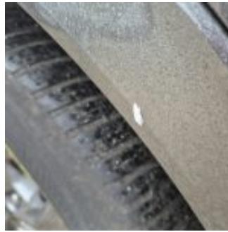
Damage Type Scratch(es)
