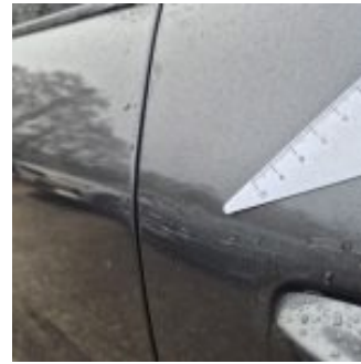
Repair Type Restyle / Touch-up
