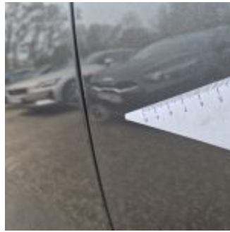
Damage Type Small dent(s)
