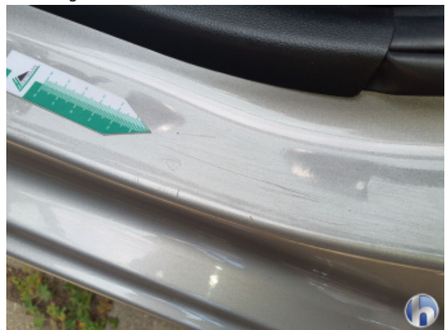
7. Schweller - Links Kratzer - Smart Repair
