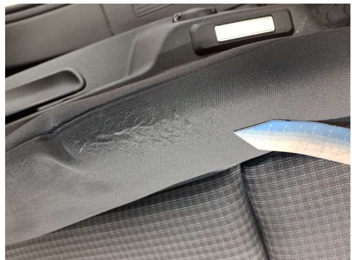
Damage 10: Seat - front: Seat cover - left side - Broken / torn - Replace
