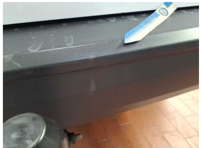
Damage 7: Rear bumper: Rear bumper (unpainted) - Scratch(es) - Loss in value
