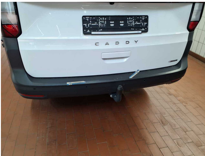
Damage 7: Rear bumper: Rear bumper (unpainted) - Scratch(es) - Loss in value
