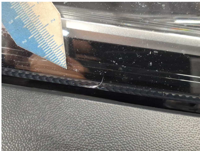
Damage 13: Headlight: Headlight - right side - Broken / torn - Replace
