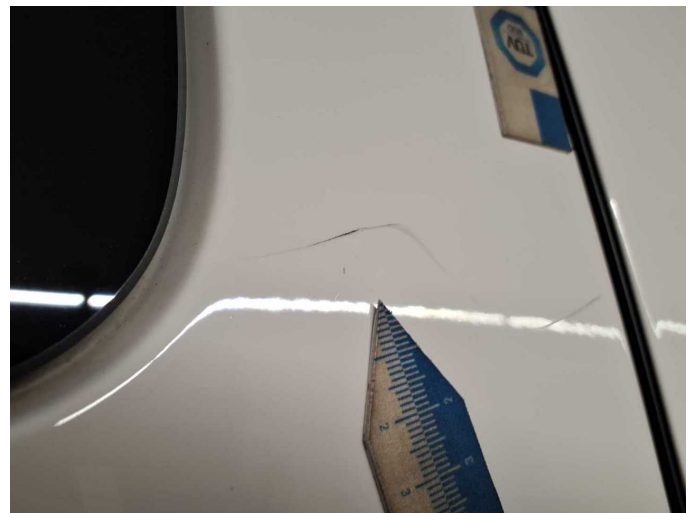
Damage 9: Sliding door, right: Sliding door with glass panel - Scratch(es) - Smart repair
