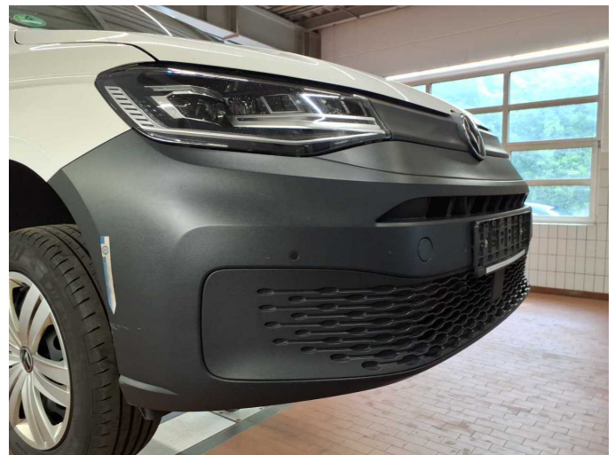
Damage 14: Front bumper: Front bumper (unpainted) - Scratched - Replace
