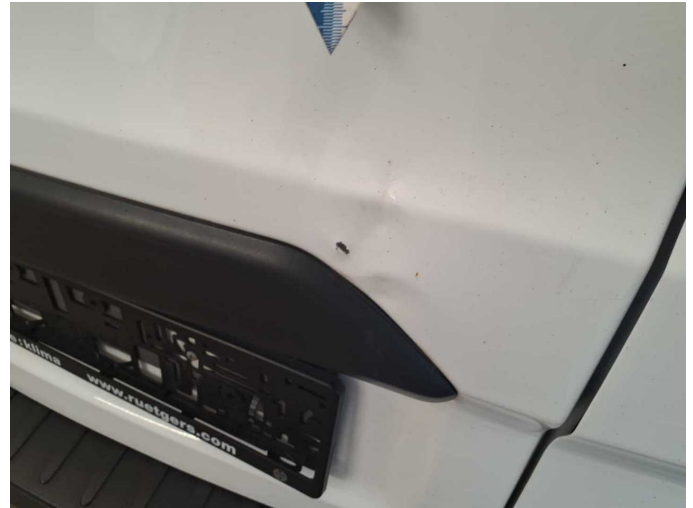
Damage 5: Boot lid / rear door: Rear door - left side (& Lackschaden) - Deformed - Repair and paint
