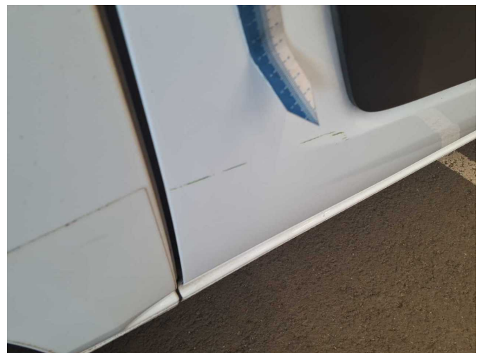
Damage 4: Sliding door, right: Sliding door - Scratched - Paint
