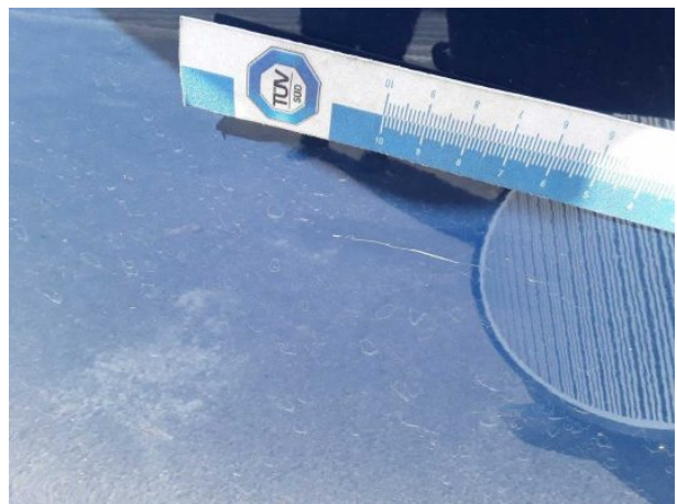
Damage 10: Door - front left side: Door - Scratched - Paint
