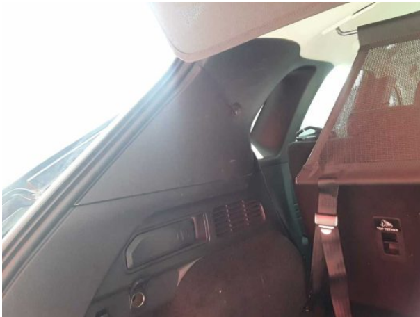
Damage 2: Trim / covers: C-pillar - trim - interior, left sde - Scratched - Loss in value
