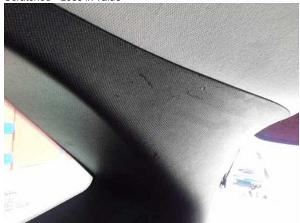
Damage 3: Trim / covers: C-pillar - trim - interior, right side - Scratched - Loss in value
