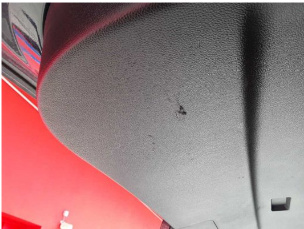
Damage 8: Trim / covers: Boot lid - interior trim - Paint defect - Loss in value
