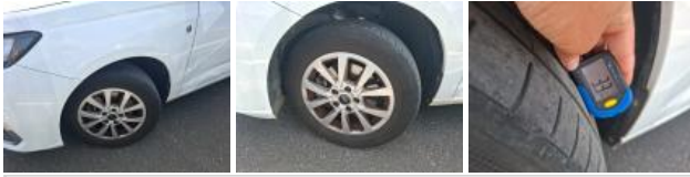
Tyre FR, Out of tolerance, Replace
