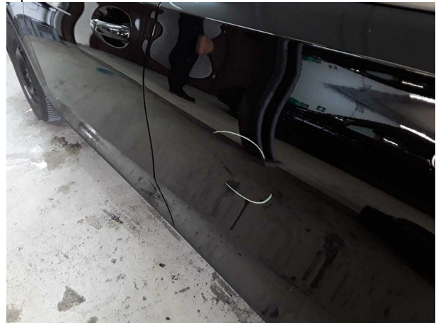
Damage #6: Door - rear left side: Door - Scratched - Repair a... paint
