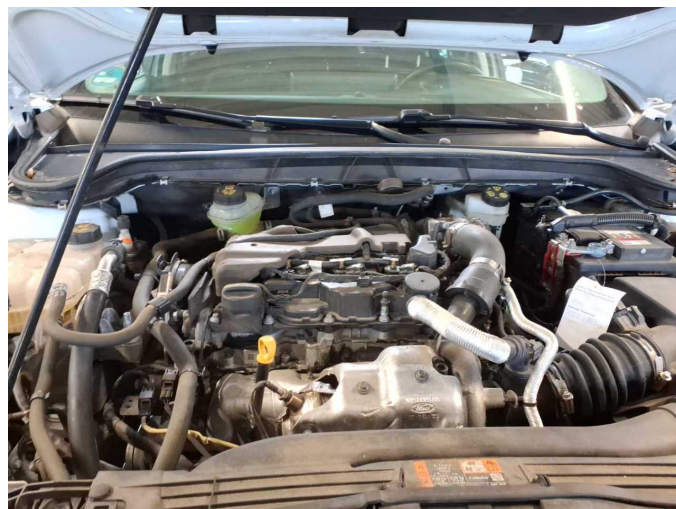
Missing part 3: Engine: Engine cover - Missing - Replace
