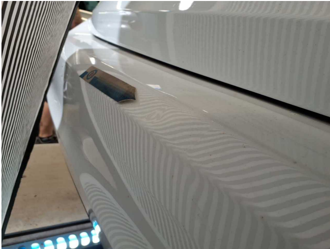
Damage 12: Rear bumper: Rear bumper - Deformed - Repair and paint
