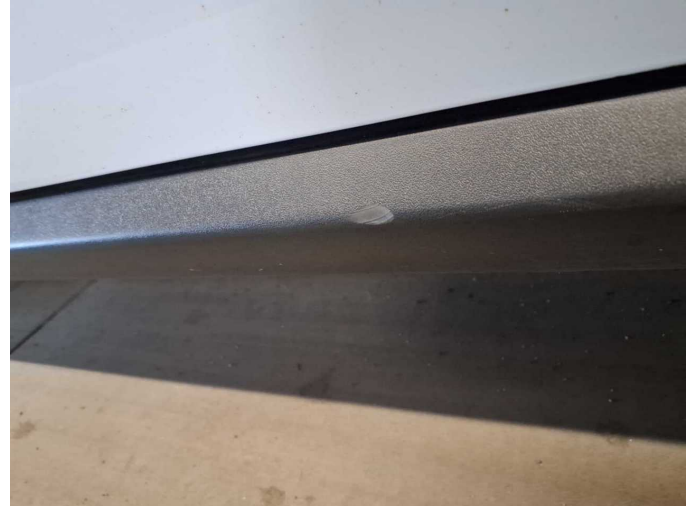
Damage 7: Sill - left side: Trim (Materialabtrag) - Scratched - Replace
