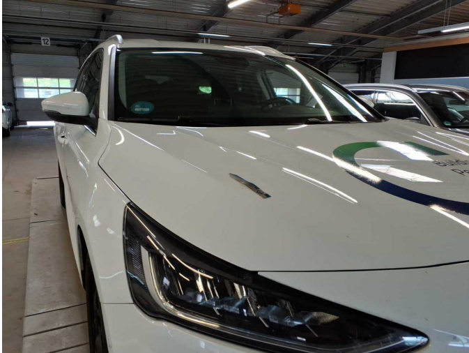
Damage 4: Bonnet: Bonnet - dent(s) - Smooth repair work
