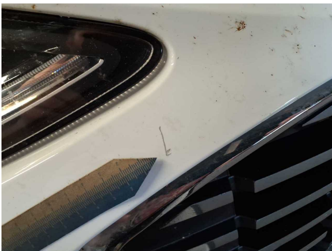
Damage 8: Front bumper: Front bumper - Scratch(es) - Smart repair
