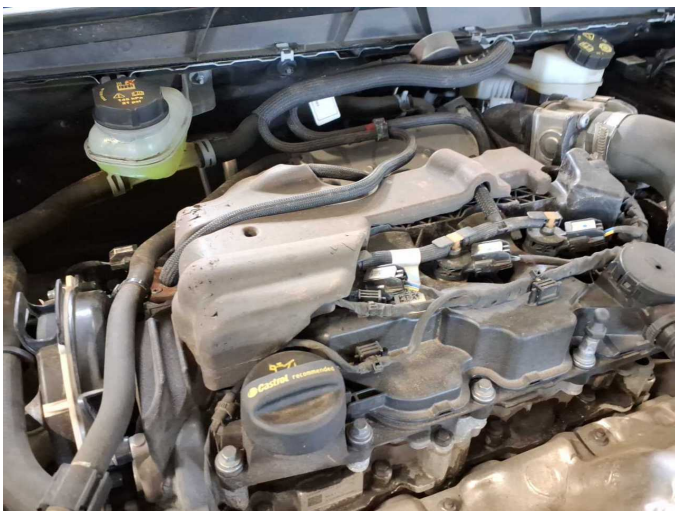
Damage 3: Engine: Engine cover (Dämmung) - Damage caused by marten / rodent - Replace
