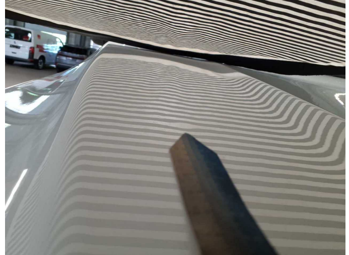
Damage 4: Bonnet: Bonnet - dent(s) - Smooth repair work
