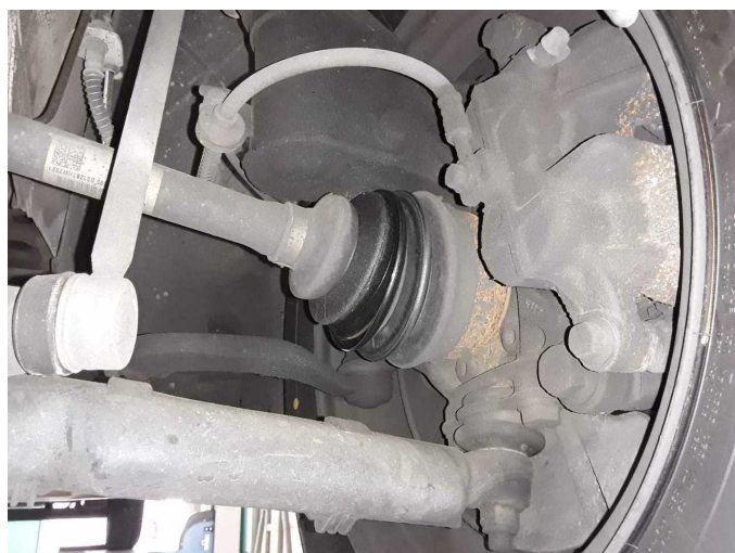
Damage 2: Drive train: Sleeve prop shaft - front left side - Broken / torn - Replace
