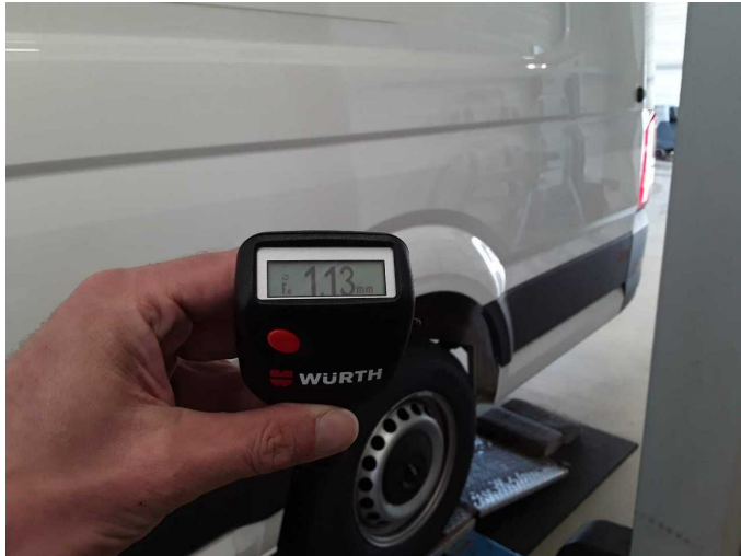
Side panel - rear left side: 1,130 µm
