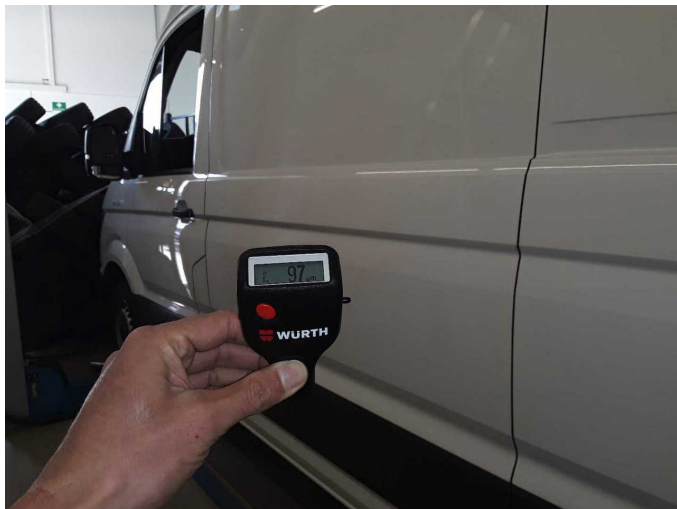
Side panel - rear left side: 1,130 µm
