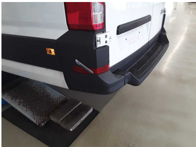
Damage 1: Rear bumper: Reflector - left side - Broken / torn - Replace
