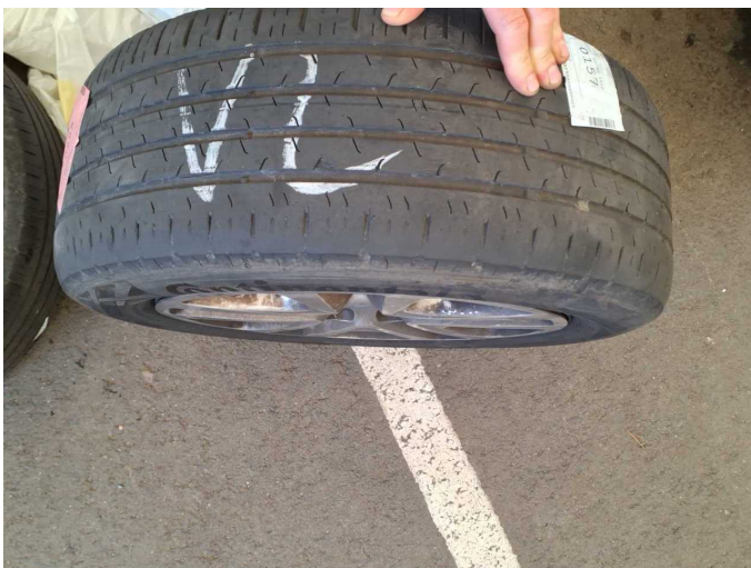
Damage 2: 2nd wheel set: 1 tyre - Worn - Replace
