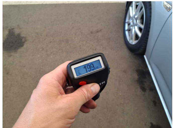
Repainting 1: Boot lid / rear door, Side panel - rear left side, Door - rear left side, Door - front left side
