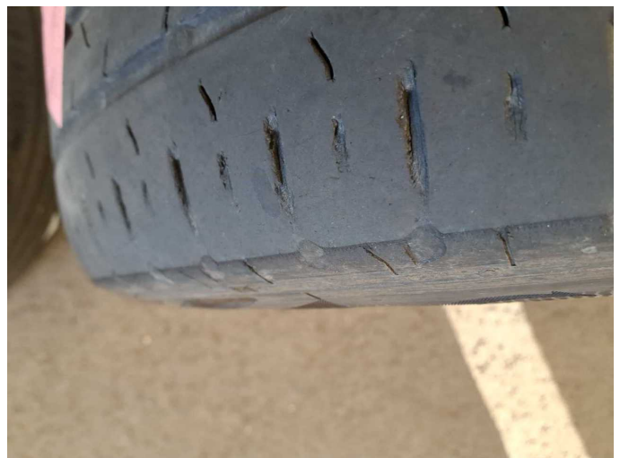
Damage 2: 2nd wheel set: 1 tyre - Worn - Replace
