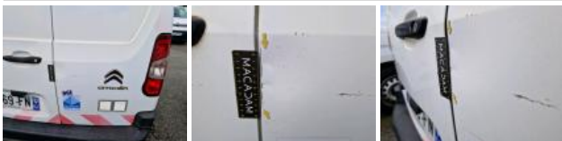
Boot door panel RL, Scratch(es), Polish
