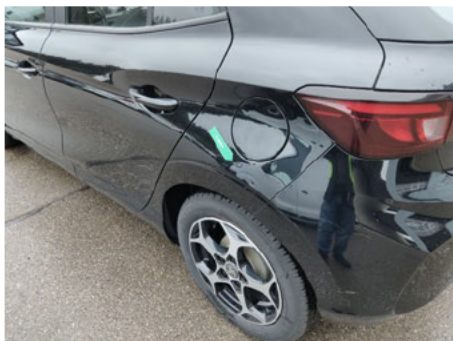
Kotflügel / Hinten Links / Delle
