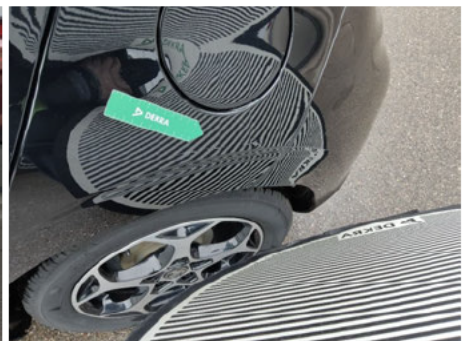
Kotflügel / Hinten Links / Delle
