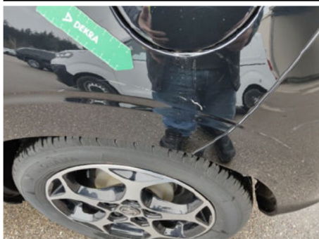
Kotflügel / Hinten Links / Delle
