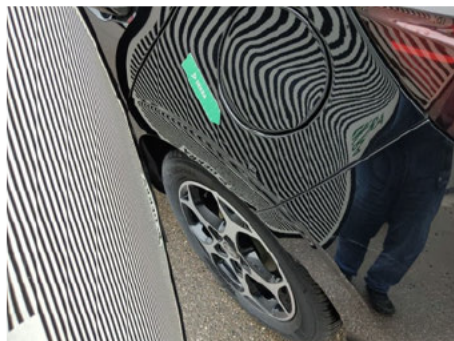
Kotflügel / Hinten Links / Delle
