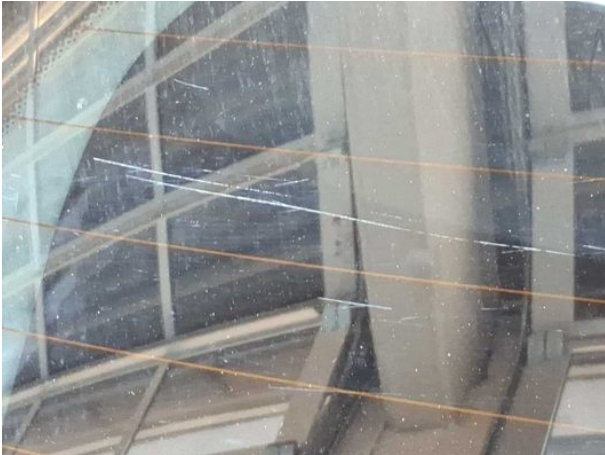
Damage #8: Vehicle glazing: Rear window - Scratch(es) - Replace
