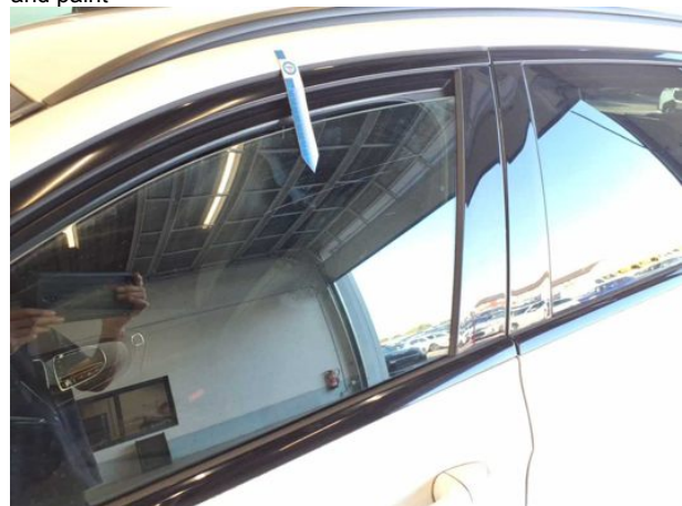
Damage #6: Vehicle glazing: Door glass - front left side - Scratch(es) - Replace
