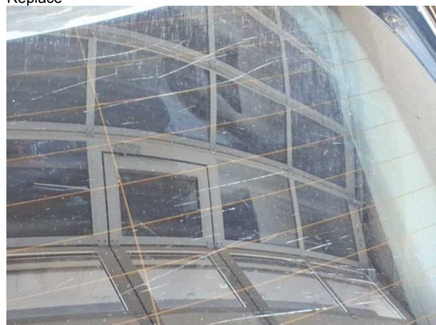
Damage #8: Vehicle glazing: Rear window - Scratch(es) - Replace
