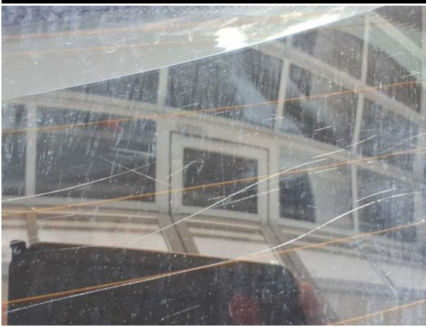
Damage #8: Vehicle glazing: Rear window - Scratch(es) - Replace
