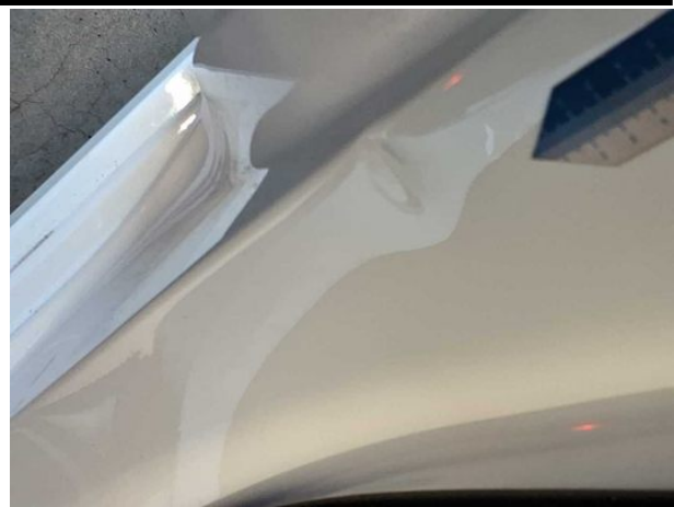
Damage #4: Side panel - rear right side: Sill - dent(s) - Repair and paint
