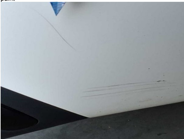
Damage #5: Rear bumper: Rear bumper - Scratch(es) - Repair a... paint
