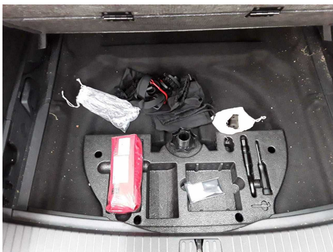
Missing part 1: Equipment: Tirefit complete - Missing - Replace
