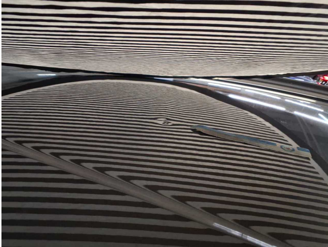
Damage 4: Roof: Roof - dent(s) - Smooth repair work
