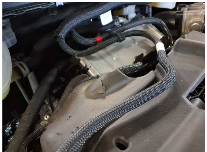
Damage 1: Engine: Engine cover (Dämmung) - Damage caused by marten / rodent - Replace
