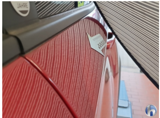
10. Tür Hinten - Links 1 Delle - Sanft Instandsetzen
