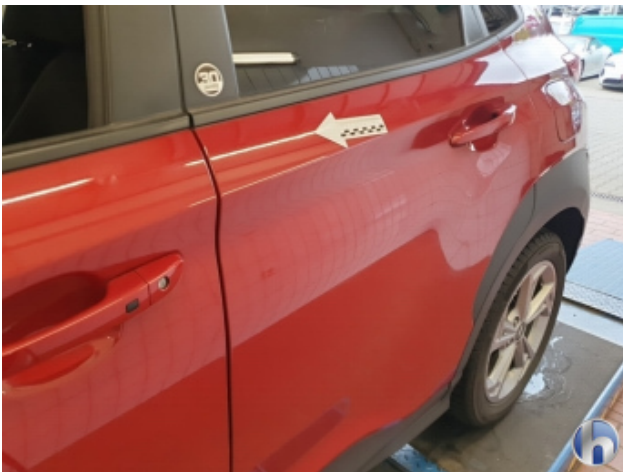
10. Tür Hinten - Links 1 Delle - Sanft Instandsetzen
