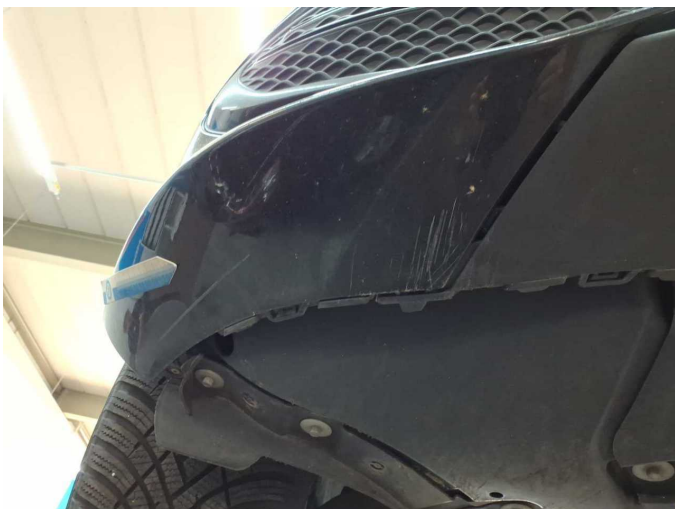
Damage 2: Front bumper: Front bumper (Und verkratzt) - Stone chips - Paint
