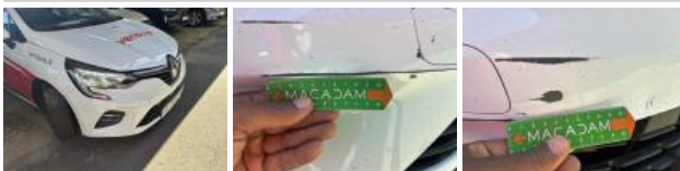
Bumper F, Scratch(es), Repair and paint (complete)
