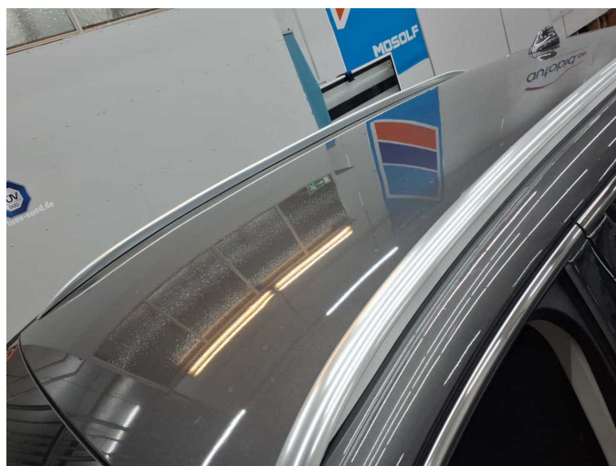
Damage 5: Roof: Roof - dent(s) - Smooth repair work
