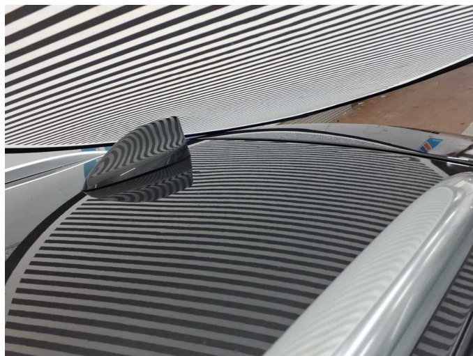
Damage 5: Roof: Roof - dent(s) - Smooth repair work
