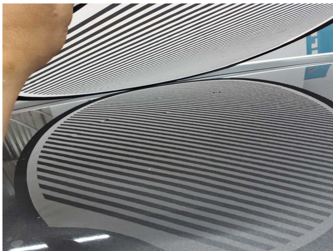
Damage 5: Roof: Roof - dent(s) - Smooth repair work
