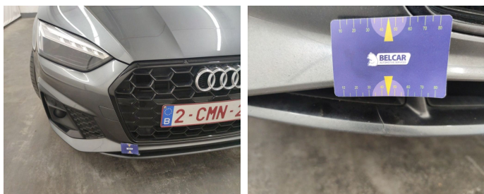
Bumper Front / Spoiler / Replace-cracked
