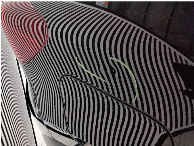
Damage 11: Side panel - rear right side: Side panel - dent(s) - Smooth repair work
