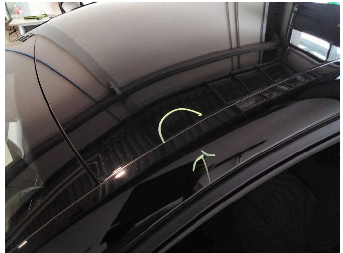
Damage 10: Roof: Roof - dent(s) - Smooth repair work
