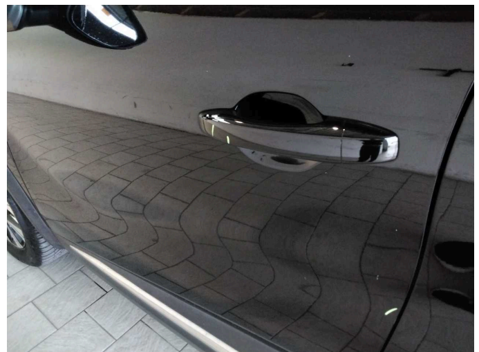
Wear and tear 1: Door - front left side: Door handle - outside - Scratch(es) - No deduction
