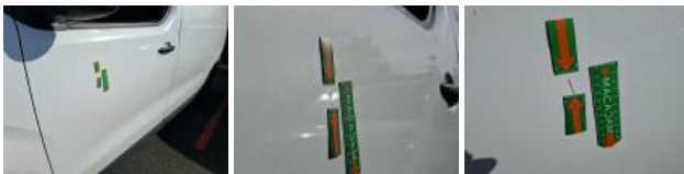
Outer sill L, Dent(s), Repair and paint (complete)
