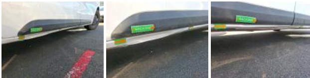
Side wall RR, Dent(s), Repair and paint (complete)
