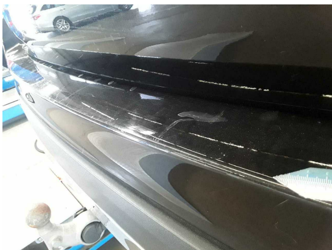
Damage 5: Rear bumper: Rear bumper - Scratch(es) - Paint
