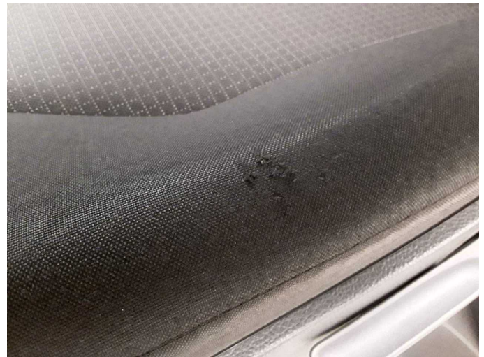
Damage 1: Seat - front: Seat cover - left side - Broken / torn - Smart repair
