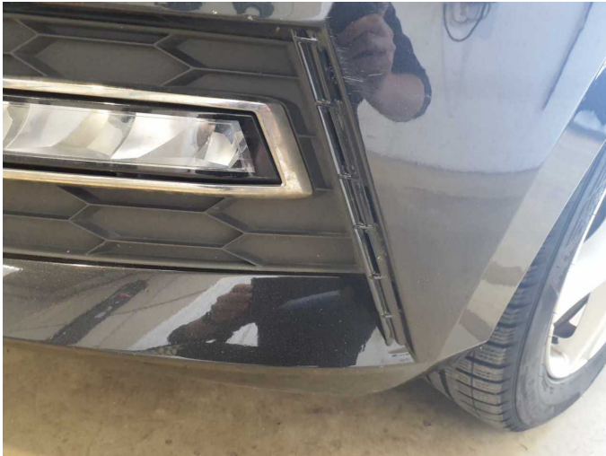
Damage 12: Front bumper: Front bumper (Inklusive Anbauteile, Nebelleuchte links gebrochen) - Dent / paintcoat damage - repair according to calculation
