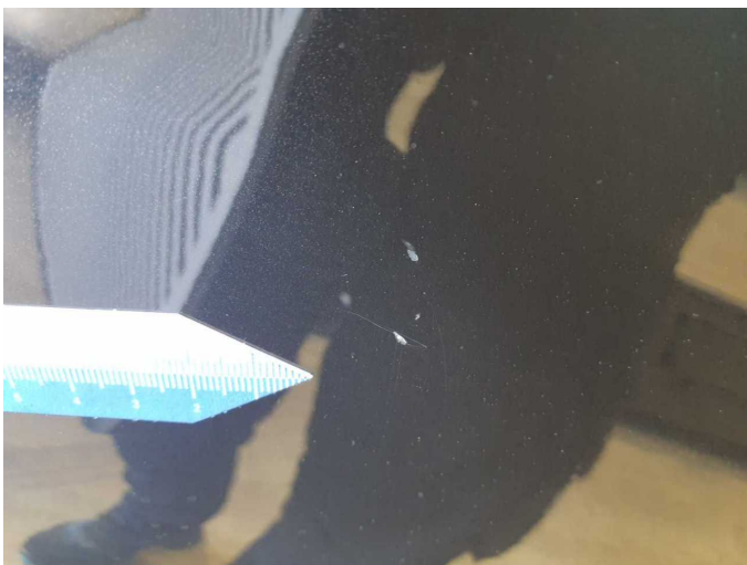
Damage 8: Door - rear right side: Door - Dent / paintcoat damage - Paint
