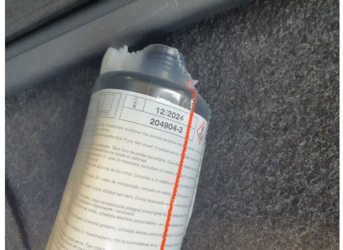
Damage 1: Equipment: Tirefit filler - Expired - Replace
