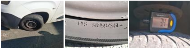
Tyre RR, Out of tolerance, Replace
