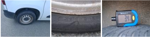
Tyre FR, Out of tolerance, Replace
