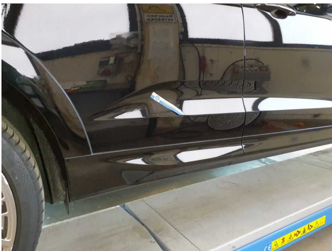
Damage 5: Door - rear right side: Door - Scratch(es) - Smart repair
