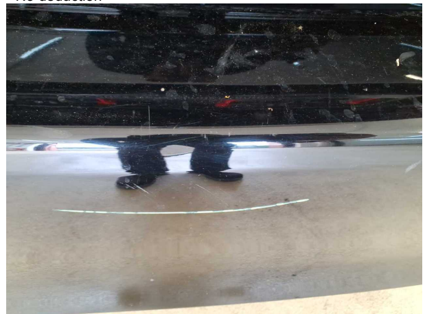
Damage #3: Rear bumper: Rear bumper - Scratch(es) - Cove... polish
