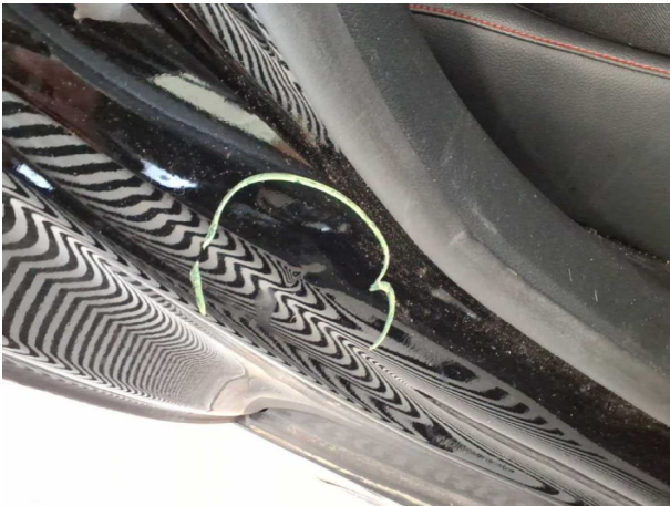
Damage #9: Side panel - rear right side: Sill - Dent / paintcoat damage - Smart repair
