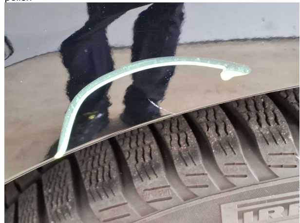
Damage #5: Side panel - rear left side: Side panel - Scratched... Cover / polish
