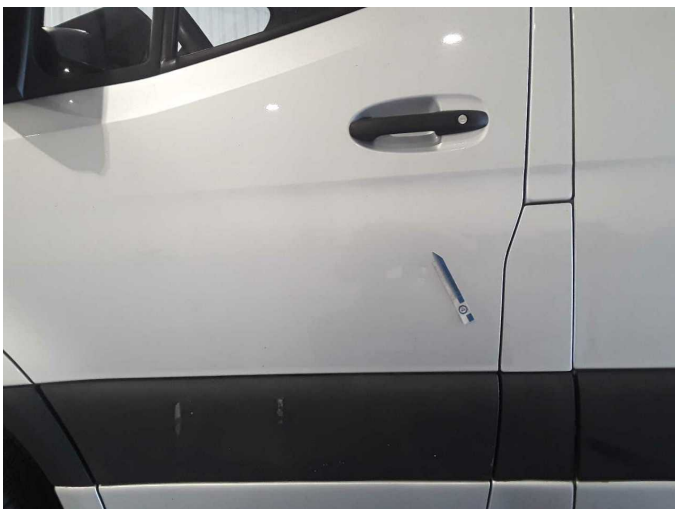
Beschädigung 14: Tür vorn links: Tür - Delle / Lackschaden - Smart Repair
