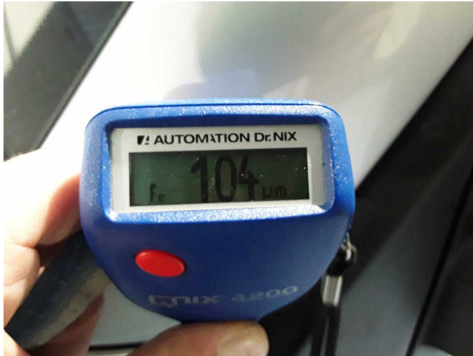
Dachholm links: 104 µm
