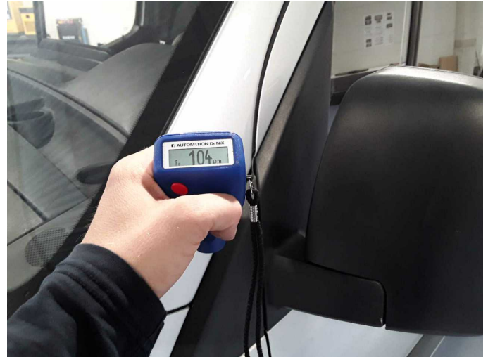
Dachholm links: 104 µm
