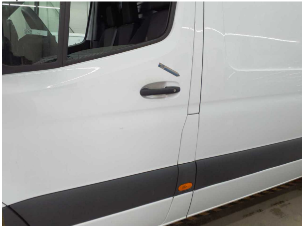
Beschädigung #13: Tür vorn links: Tür - Delle / Lackschaden - Smart Repair
