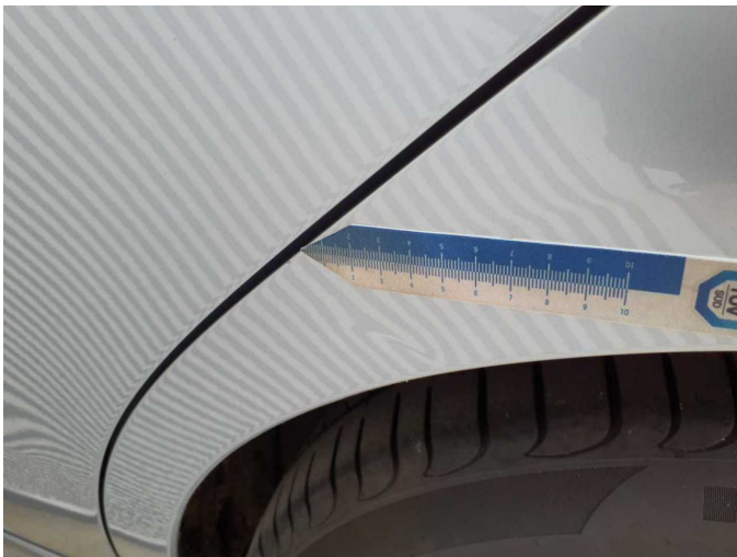
Damage 4: Side panel - rear left side: Side panel - Deformed - Repair and paint
