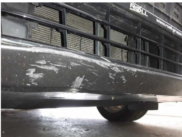
Damage #23: Front bumper: Front bumper - Deformed - Replace
