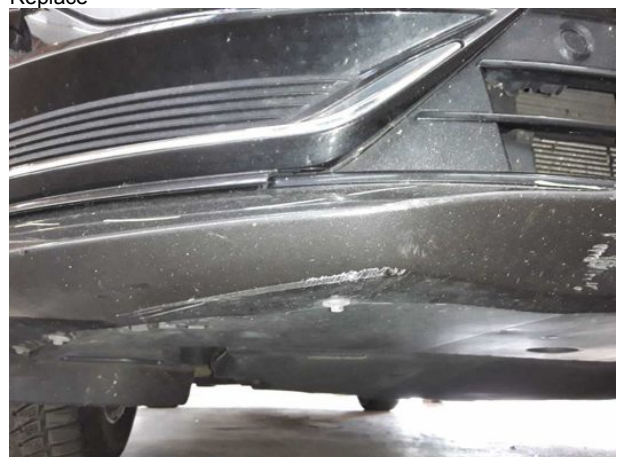
Damage #23: Front bumper: Front bumper - Deformed - Replace
