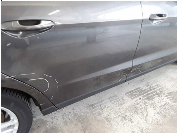
Damage #19: Door - rear right side: Door - Dent / paintcoat dama... - Repair and paint
