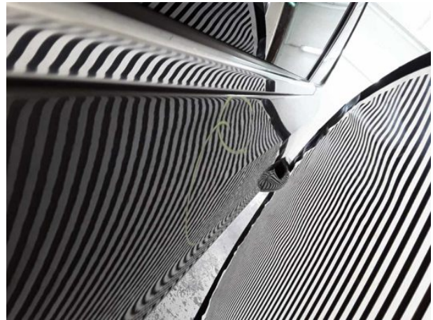
Damage #20: Door - rear left side: Door - Dent / paintcoat damage - Repair and paint
