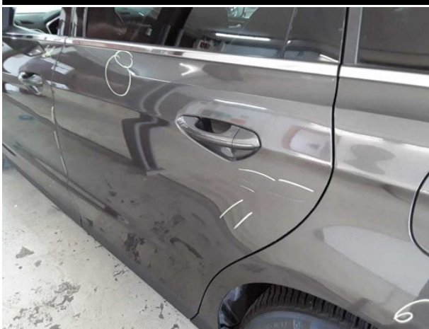
Damage #20: Door - rear left side: Door - Dent / paintcoat damage... Repair and paint
