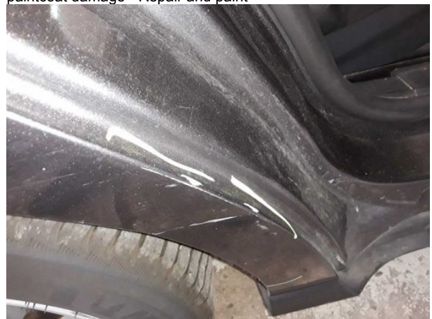
Damage #21: Side panel - rear right side: Side panel - Dent / paintcoat damage - Repair and paint
