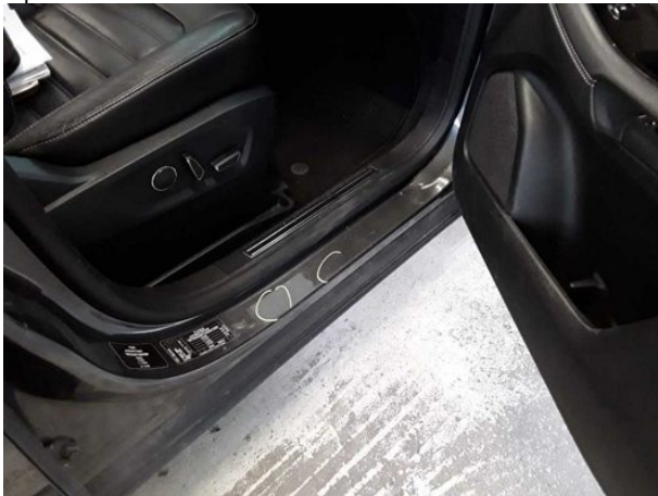
Damage #13: Sill - right side: Sill - dent(s) - Smooth repair work
