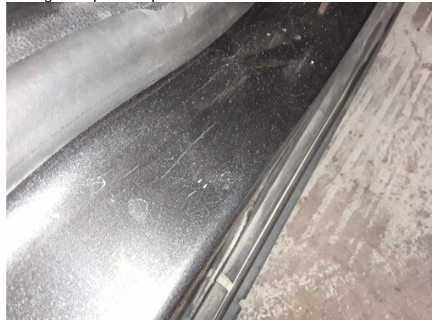
Damage #15: Side panel - rear right side: Sill - Dent / paintcoat damage - Repair and paint
