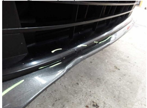
Damage #23: Front bumper: Front bumper - Deformed - Replace
